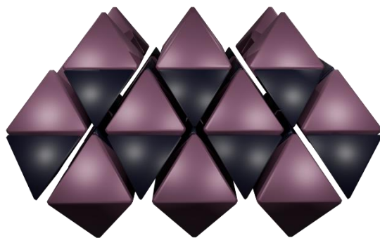
Figure 4.1. Schematic illustration of the tetrahedral-octahedral honeycomb (TOH) structure.
