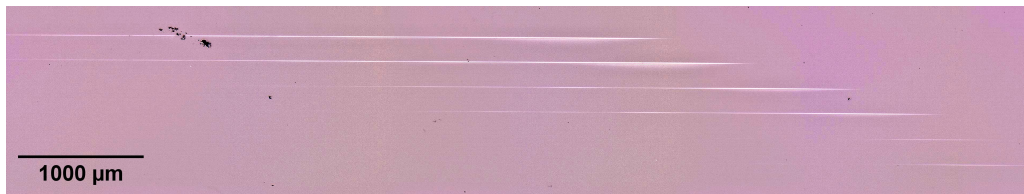
Figure 4.25: Representative single-shot damage craters at 1keV photon energy at 9 mrad incident angle for Si without coating.
