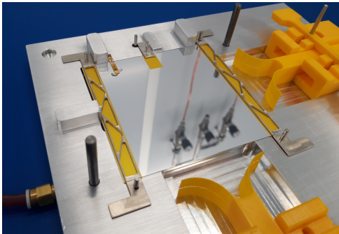
(c) Bare module integration
