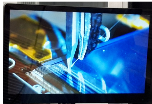
(f) Wire bonding process
