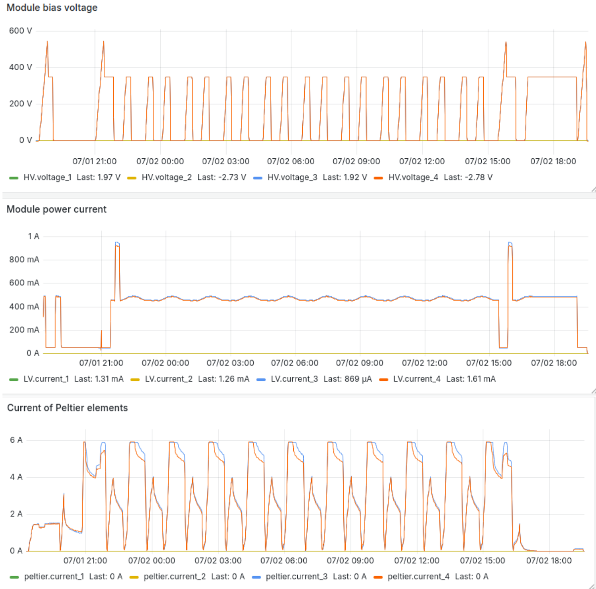
Figure 3.41: Grafana display with plots from successful thermal cycling of two modules on chucks 3 and 4. The plots of the module bias voltage, the current powering the modules, and the current in the Peltier elements are shown.
