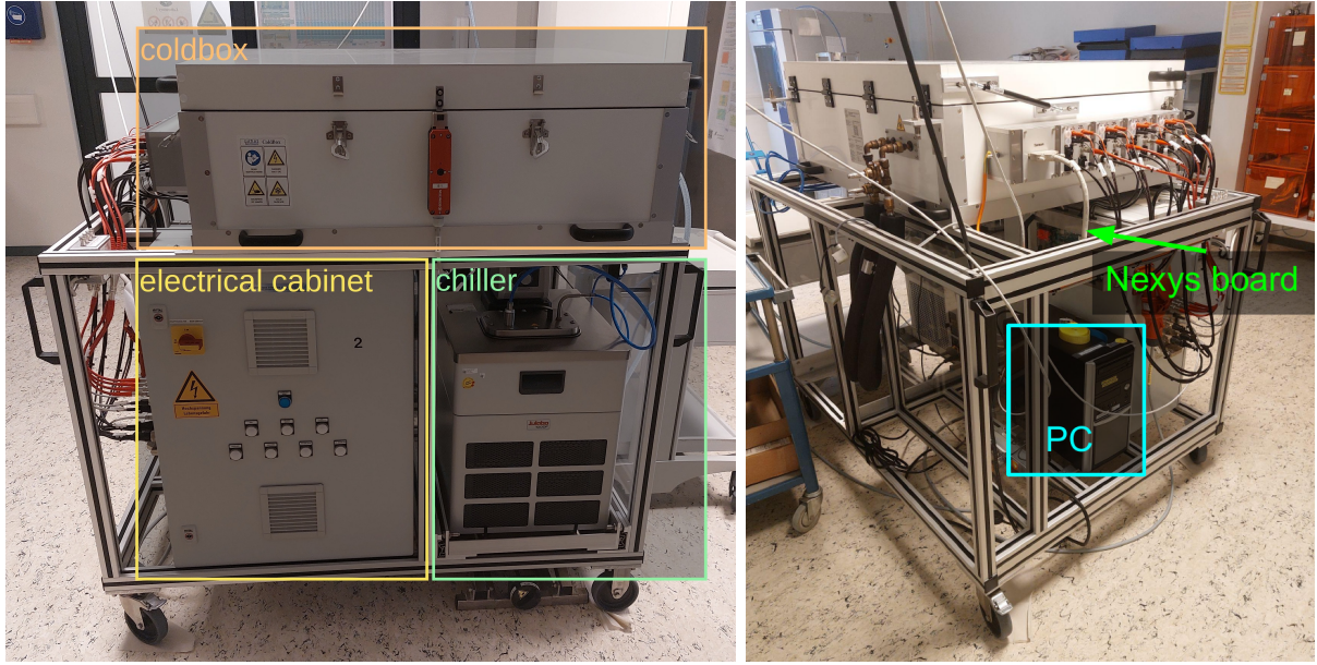
Figure 3.32: The main components of the thermal cycling setup.
