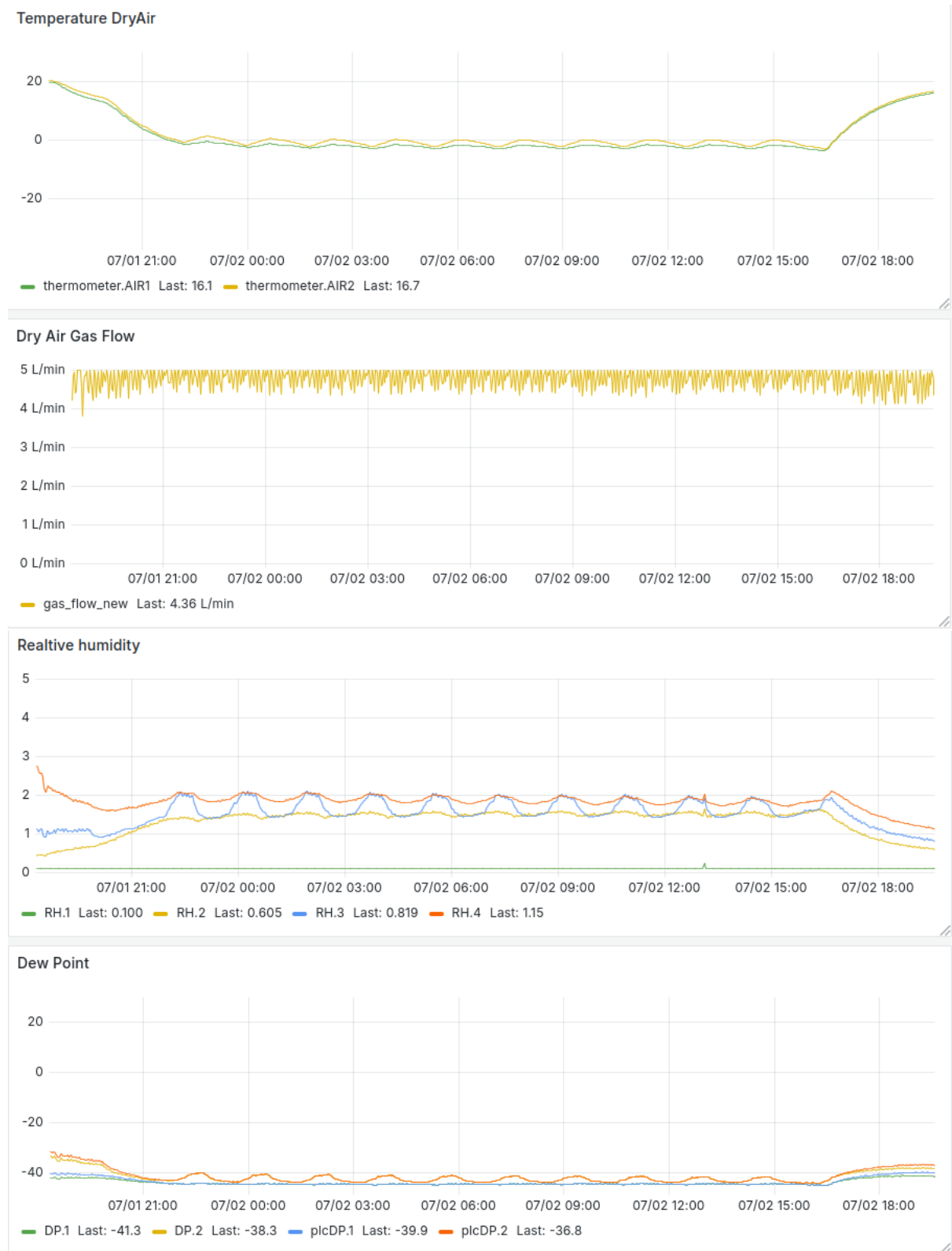
Figure 3.40: Grafana display with plots from successful thermal cycling of two modules on chucks 3 and 4. The plots of the temperature of dry air at the output from the modules, the flow of dry air, relative humidity, and the dew point are shown.
