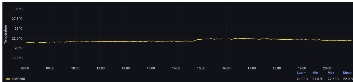
Figure 6.5: Measurement of ambient temperature in the laboratory extending over 12 h. The data was taken with a Bosch BME280 sensor [87].
