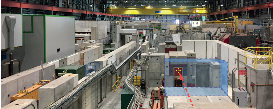
Figure 8.2: Downstream view along the H6 beamline into zone B. The photograph of the empty zone B was taken from above the open beam stop of H6A, as marked in Figure 8.1. A yellow cross on the red metal block marks the position of the impinging beam, the red arrow. The placement of the telescope setup is traced by a light blue cube.
