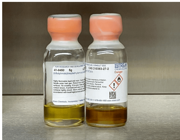
Figure A.4: Two different TBTDEN bottles showing substantial discrepancy in colour. Both are 5g of minimum 98% purity TBTDEN however, their colour is notably distinct.
