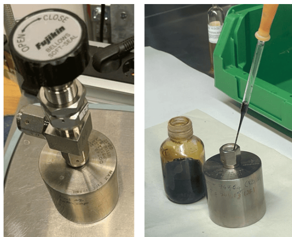
Figure A.3: Photographs: left a precursor container from the system GEMStar XT-DP TM and right decomposed precursor (handle in a controlled atmosphere inside of a glove box).
