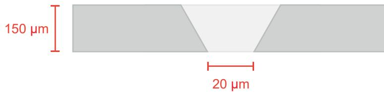
Figure 4.7: Schematic of sapphire shadow mask for  $C_{60}$  growth.
