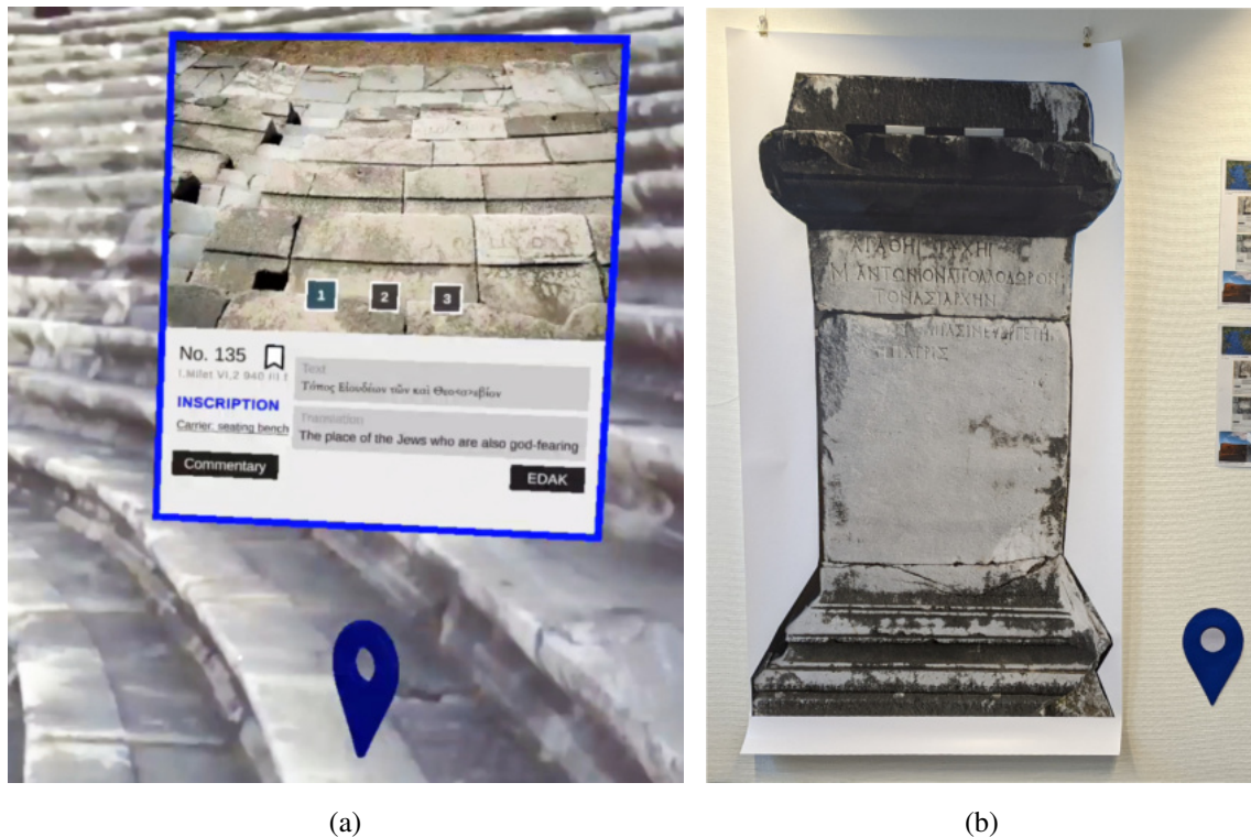
Figure 4.21: Testing MR prototypes for visualizing spatial information panels in real-life settings: (a) Nreal Light application with 3D marker and info panel captured at the theater of Miletus and (b) HoloLens 2 application with 3D marker and almost true-to-scale WA printout.
