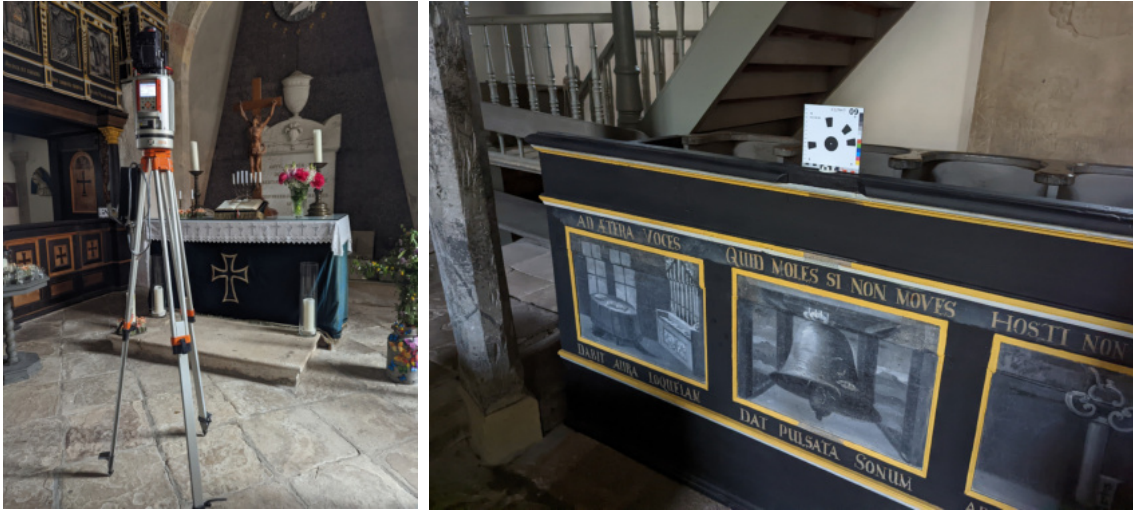
Figure 3.3: (Left) 3D LIDAR scanner and (right) coded target used as references in the scanning process by ArcTron 3D.
