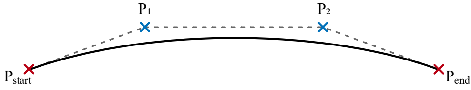
Figure 6.4: Illustrated cubic Bézier curve configuration for RayCurve and RayCurveRotation .
