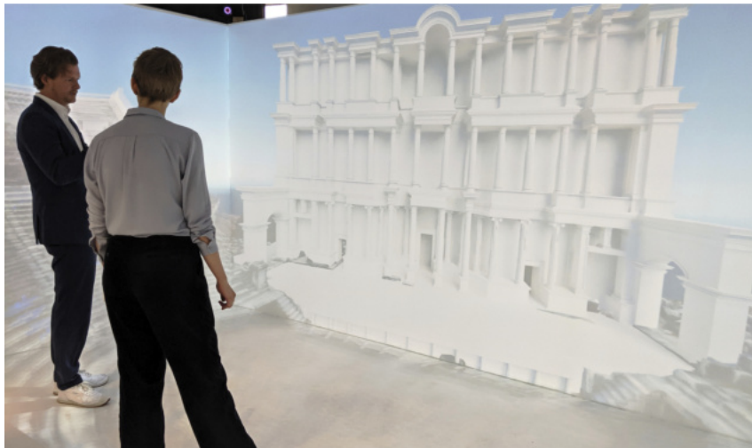
Figure 4.19: CAVE in monoscopic view mode without positional tracking of the user, allowing multiple users to join the experience (projection shows the reconstructed stage of the theater).
