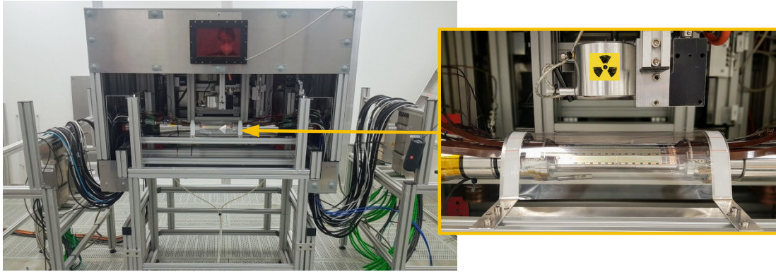
Figure 7.12.: PXD half-shell test setup at DESY with the front panel opened. The magnified region highlights the source holder positioned above a PXD half-shell mounted on the Al BP mockup. A 50 \mu\text{m} thick polyethylene (PE) foil covers the half-shell to protect it from abrasions caused by the source holder mechanics.
