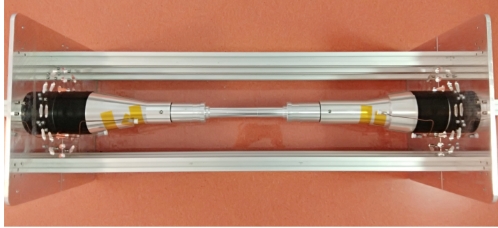
Figure 7.4.: The Al BP mockup was already utilized for the PXD1 commissioning. The thin, round section at the center represents the mockup of the actual beryllium (Be) component that covers the IP. This central section is enclosed by the PXD. The mockup BP is surrounded by Al profiles, which are mounted together with the mockup BP onto two end plates that support the entire setup.
