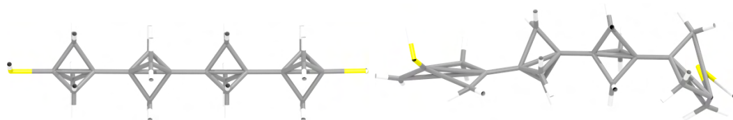
Figure 6.21: The 4-staffane-3,3'-dithiol molecule (left) is inadequately represented by the ReaxFF, resulting in rapid decomposition (right).
