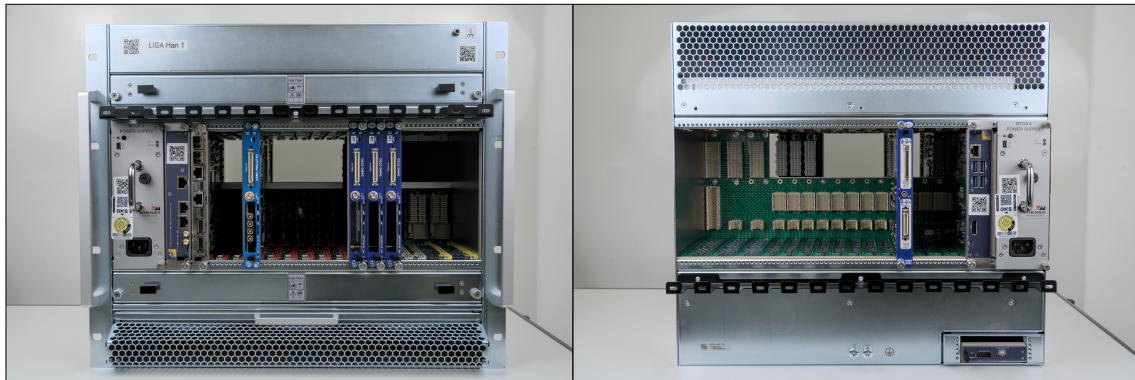
Figure G.2: Pictures of a partially filled "NATIVE-R9" (MTCA) Crate. The left picture shows the front side and the right the back side of the crate. From left to right of the front side one can see: the PSM, the MCH, an XYA AMC module, two empty slots, the "z7io" AMC module I use, 5 more open slots, and after 3 more "z7io" AMC modules. In the rear / back side, from left two right are: the PSM, the MCH, empty slots, and a single RTM connected to the z7io" AMC that I use.
