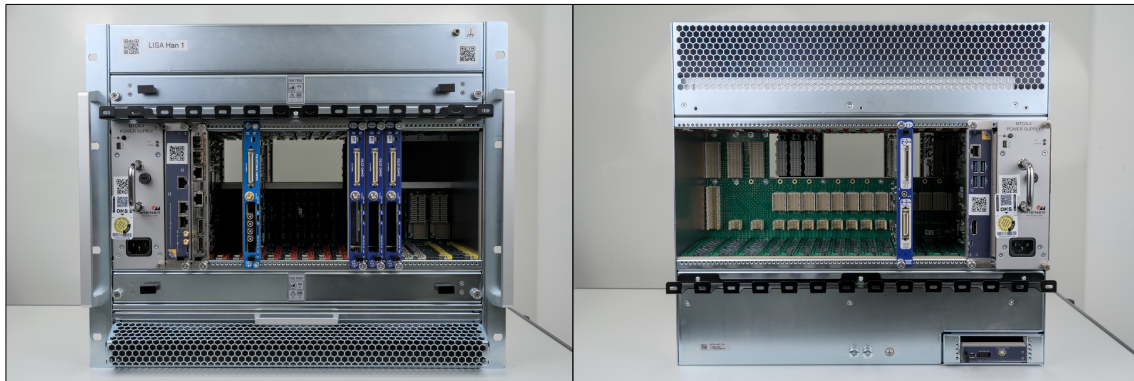
Figure 10.6: Pictures of a partially filled “NATIVE-R9” (MTCA) Crate. The left picture shows the front side and the right the back side of the crate. From left to right of the front side one can see: the PSM, the MCH, a “CPU” AMC module, two empty slots, the “Z7IO” AMC module I use, 5 more open slots, and then 3 more Z7IO AMC modules. In the rear / back side, from left to right are: the PSM, the MCH, empty slots, and a single RTM connected to the Z7IO AMC that I use.
