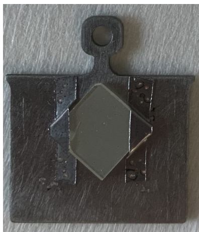
Figure 4.3: Rutile \text{TiO}_2(110) single crystal mounted with Ta clips on a Mo sample holder.
