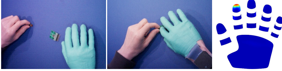
Figure 5.7.: Camera images (left, middle) and tactile data (right) for an assembly task.
