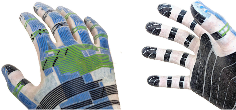
Figure 4.28.: Partially finished sensor glove on a human hand, with sensor elements and conductor bundles transferred to the glove surface. A subset of conductive traces is colored in green and blue for easier identification [296].
