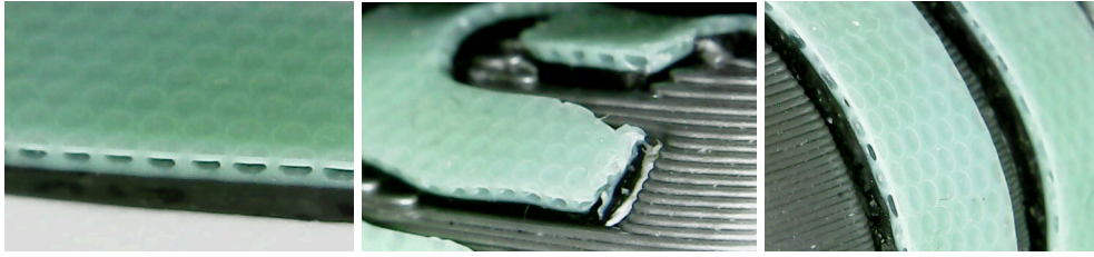
Figure 4.13.: Closed-celled dielectric structures after casting (left [292]) and on fixtures for sensor assembly (middle [292], right).
