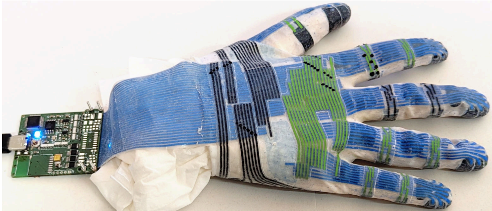
Figure 4.29.: Tactile sensor glove during assembly with attached readout board for diagnostics [296].
