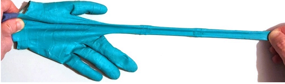
Figure 4.33.: The teaching glove, including conductors and sensors, is completely made from highly stretchable silicone rubber [296].
