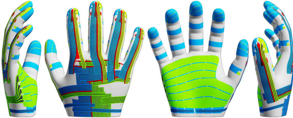
Figure 4.26.: CAD model of a tactile sensor glove [296]. Electrodes for sensor rows and columns are shown in green and blue, spacing constraints in black and ground electrodes in red.
