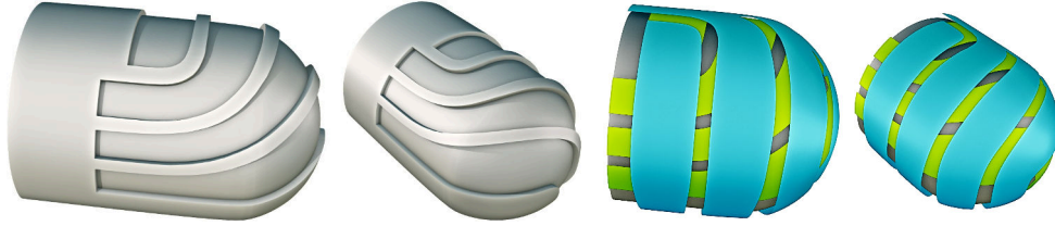
Figure 4.21.: Assembly fixture (left) and electrode layout (right) for a double-curved fingertip sensor [292].
