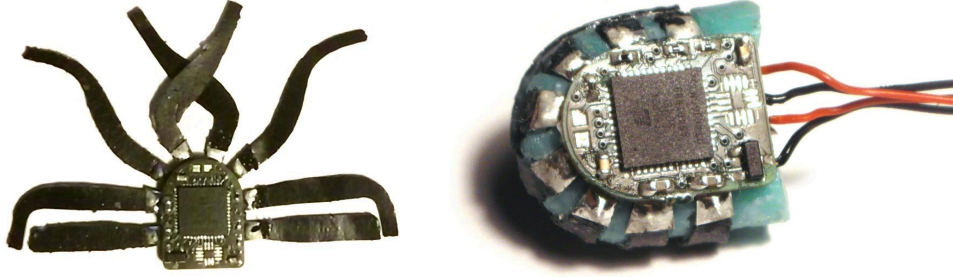
Figure 4.22.: Silicone electrodes are soldered via metal tabs to a finger-nail readout board (left) and assembled into a double-curved wearable fingertip sensor (right) [292].
