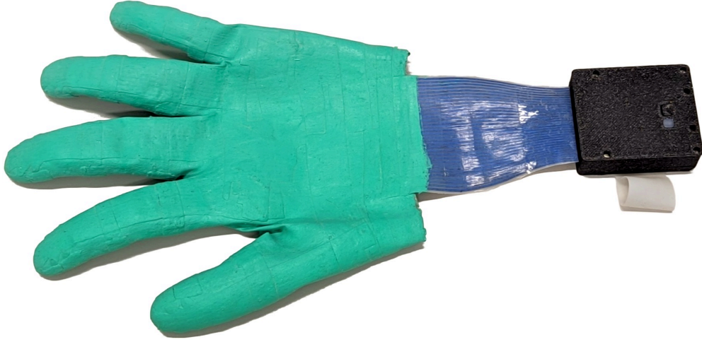
Figure 4.30.: Fully assembled tactile sensor glove [296].
