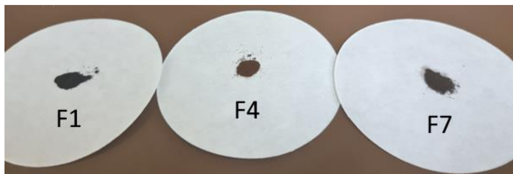
Figure 2. Humins obtained from fructose in different solvents using sulfuric acid as strong Brønsted acid.
