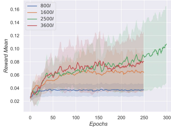
Figure 6.12: The learning curves of our RL agent for representation are trained from different gain matrices in the impedance controller.
