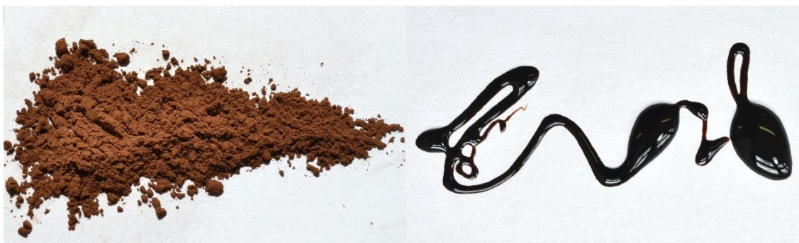
Figure 2. Unmodified solid lignin before and liquid lignin-containing polyol after oxypropylation.
