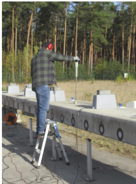
Figure A.5: The triggering of the Vertical Impulsive Source on the North span bridge (by BAM)
