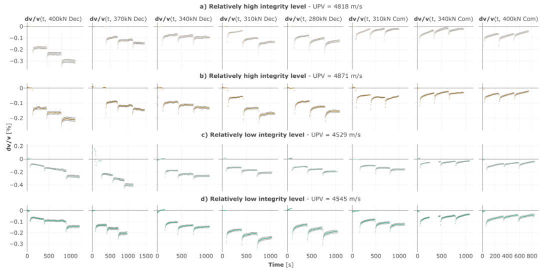
Figure 3.1: Datasets recorded at the four locations of the bridge at eight different compressive force levels. a) Plots of the eight datasets recorded on the south-left side. This side is categorised as concrete with a relatively high integrity level due to the high ultrasound pulse velocity values. b) Plots of the eight datasets recorded on the south-right side (a side with a relatively high integrity level). c) Plots of the eight datasets recorded on the north-left side. This side is categorised as concrete with a relatively low integrity level due to the low ultrasound pulse velocity values. d) Plots of the eight datasets recorded on the north-right side (a side with a relatively low integrity level).
