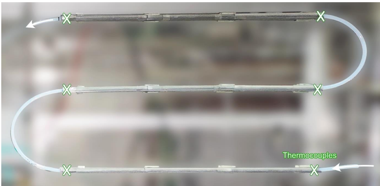
Figure 10: Photograph of RV 4, where three assembled reactor sections are in one level, and there are three total levels between which the PTFE tubing is bent.
