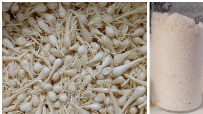
Figure 65: Polymer obtained after precipitation using a too concentrated polymerizate (left) and using optimum conditions (3% s.c., right).
