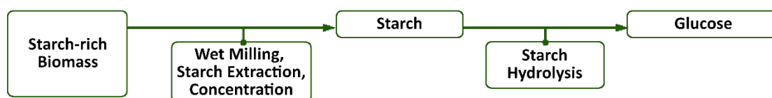
Figure 9: Schematic overview of the processing steps for starch-rich biomass. Adapted from Witzke. [25]
