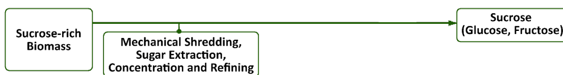
Figure 7: Schematic overview of the processing steps for sucrose-rich biomass. Adapted from Witzke. [25]
