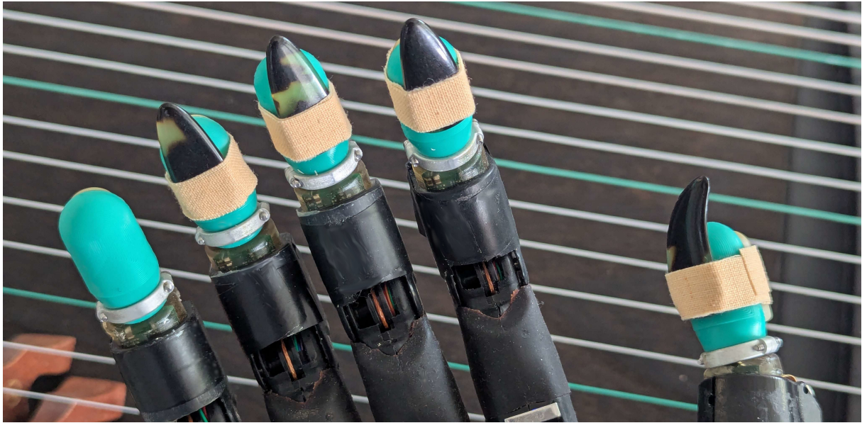
Figure 4.2 – Close-up view of the Shadow Hand fingertips with SynTouch BioTac tactile sensors (turquoise), prepared with traditional fingernail plectra for Guzheng playing. Each plectrum is taped to the fingertip to reach several millimeters beyond the tip with stable contact to the sensor surface. The thumb is taped with a regular curved thumb plectrum for a more relaxed hand posture during playing; little finger without a plectrum, as traditional in Guzheng playing.
