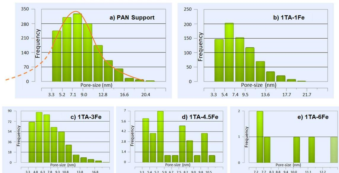
Figure S8. Pore size distribution of the porous PAN support and TA- $\text{Fe}^{3+}$  membranes fabricated at different tannic acid to  $\text{FeCl}_3 \cdot 6\text{H}_2\text{O}$  weight ratio.
