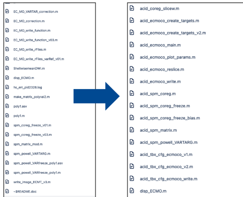
Figure 14: Example of renamed files which are part of the ACID toolbox. In the left panel, the old unstructured filenames are displayed. In the right panel, the renamed files are shown. A structured naming system is implemented based on “acid” as a prefix followed by the module name the file is contributing to (e.g., ecmoco, or tbx_cfg for main files).
