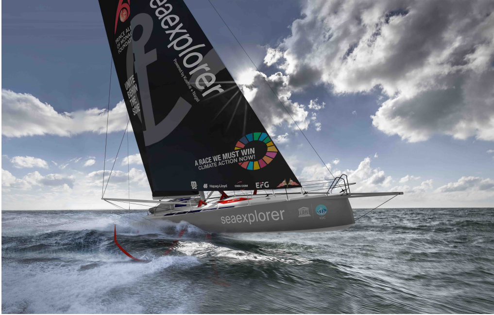
Figure 1.1: The IMOCA 60 sailboat Seaexplorer – Yacht Club de Monaco (formerly Malizia ) from Team Malizia. The IMOCA 60 is a high-performance, 60-foot (18.28 m) monohull class designed for single- or double-handed offshore racing, known for its use in round-the-world regattas such as the Vendée Globe and The Ocean Race . Since 2018, Team Malizia has collaborated with the Max-Planck-Institute for Meteorology to measure surface ocean f\text{CO}_2 during races and transfers. (Photo credit: Andreas Lindlahr).
