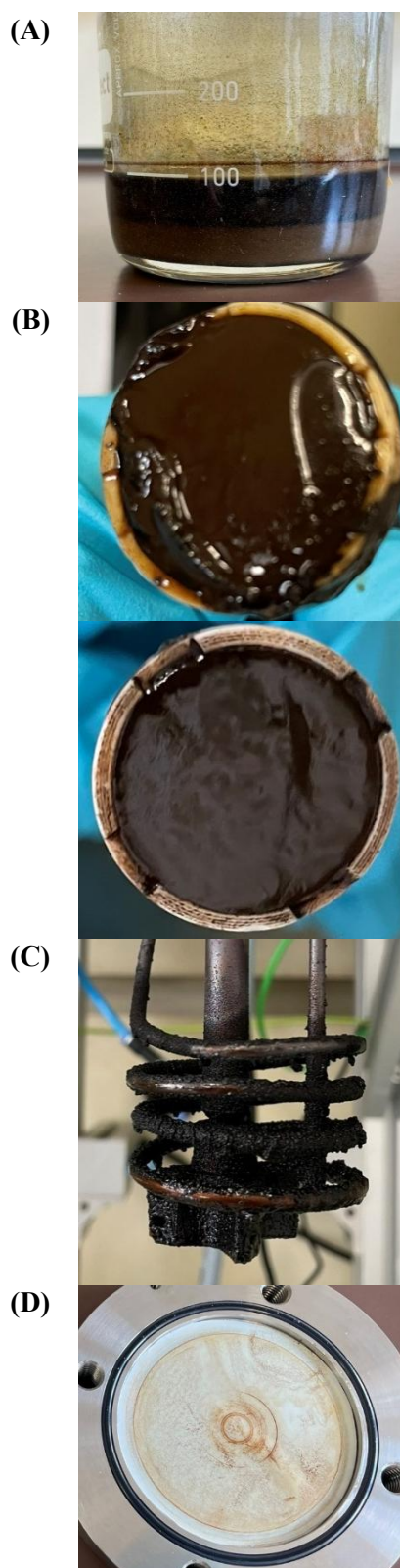
Figure 7-42: Representation of precipitation formed during continuous depolymerisation of kraft lignin S19. (A) shows the liquid product container T4, (B) shows the particle filter of the membrane module inlet side before and after cleaning, (C) shows the stirrer and cooling coil inside the reactor, and (D) the membrane sheet.
