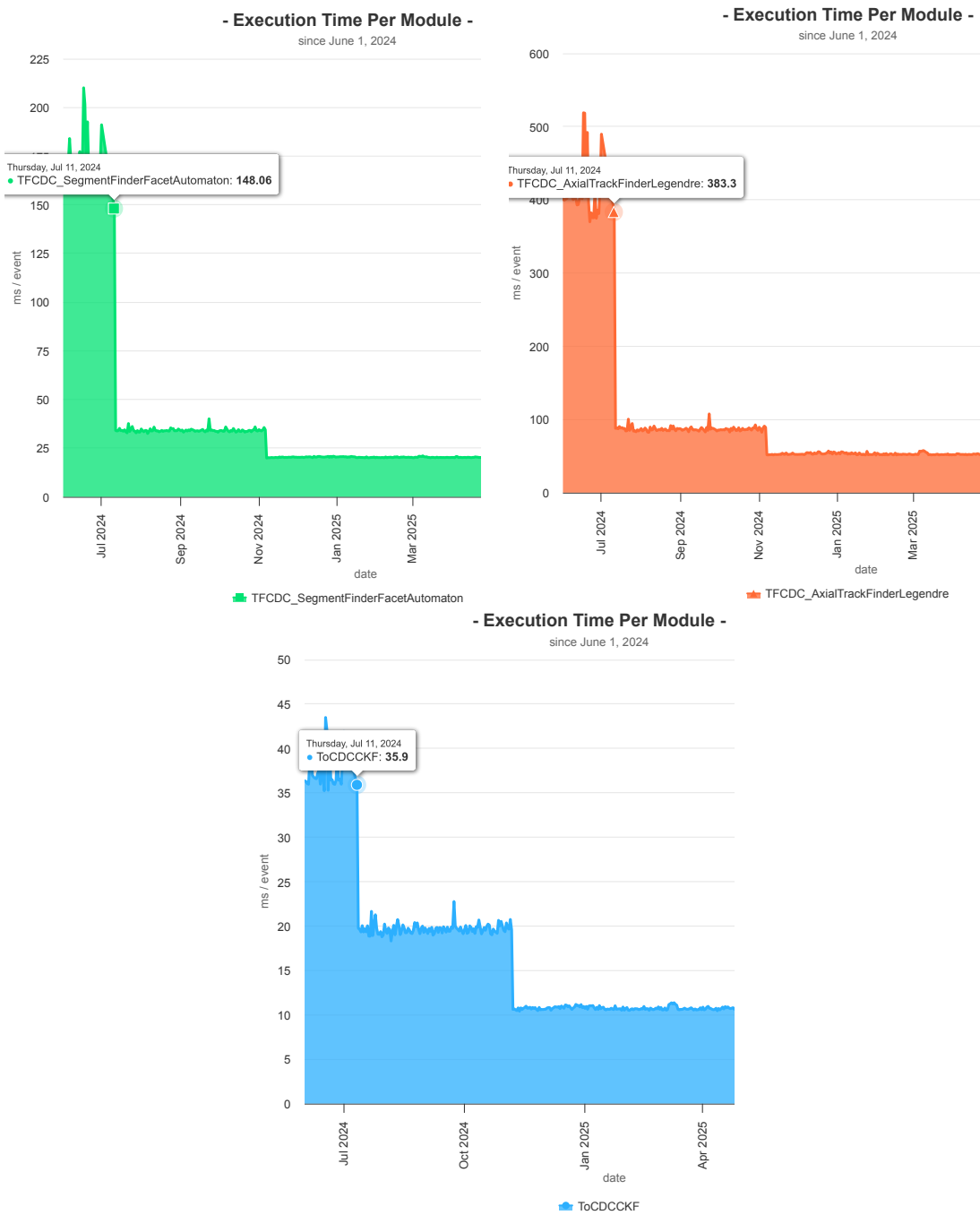
Figure 6.35: Average per-event runtime of key tracking modules before and after the MVA-based CDC background filter was introduced in Release 9. Upper left: TF CDC_SegmentFinderFacetAutomation; Upper right: TF CDC_AxialTrackFinderLegendre; Bottom: ToCDCCKF. All show substantial reductions in execution time.
