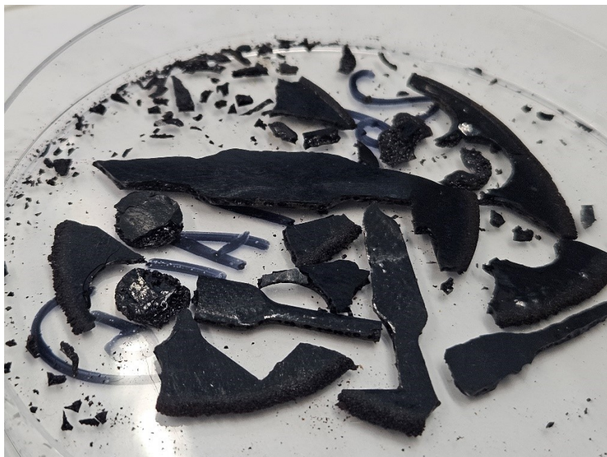
Figure S30: Lignosulfonate-based vinyl urethane vitrimer crosslinked with Priamine™ 1073. Weight ratio of lignosulfonate exceeds 55 wt.% and therefore the inhomogeneous sample is too brittle to be processed. Cutting out the samples for tensile testing and DMA only led to the shattering of the film into smaller pieces.
