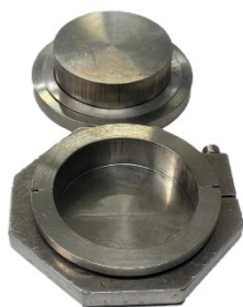
Figure S1: A heat compression mold with a diameter of 5 cm was used for the reprocessing of the vitrimers.
