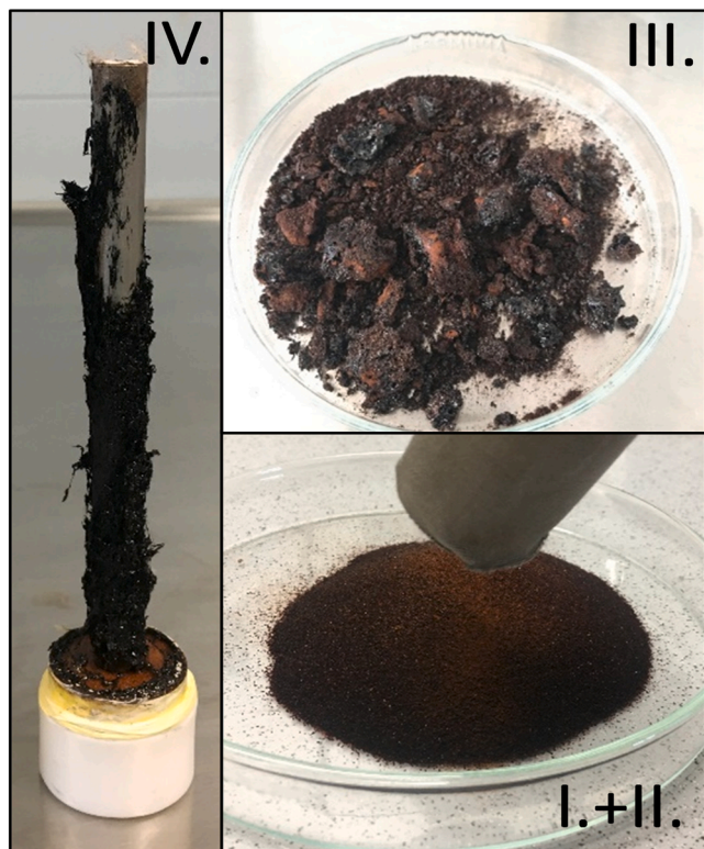
Fig. 10. Residues after the extraction of old SPL (I. + II. Adsorbed SPL, 4 h, III. Liquid SPL, 4 h, IV. Liquid SPL, 2 h).
