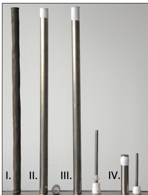
Fig. 5. Different extraction vessels (I. = Steel mesh basket, II. = Tube with mesh cap, III. = Long Tube with plug, IV. = Short Tube with plug).
