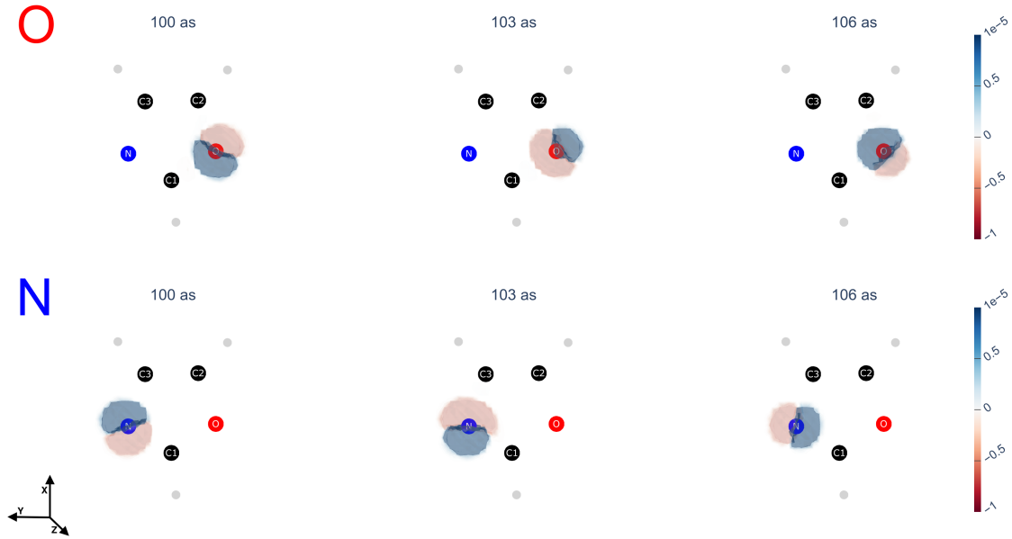
Figure 5.8: Snapshots of \rho_{\Delta}(\mathbf{r}, t) relative to the excitation with a right-handed, circularly polarised pulse in the \sigma_{xy} plane. The upper panel is relative to the excitation at the O K-Edge, the lower panel to the excitation at the N K-Edge. The orientation of the axes is illustrated in the lower left corner.
