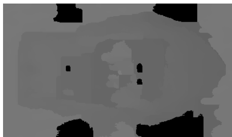
Figure 6.6 – A depth image of the same area as in Figure 6.5 taken with the Intel RealSense D405. While the printed layer is clearly visible on the RGB image, the depth image is very noisy, and the object can only be vaguely recognized.
