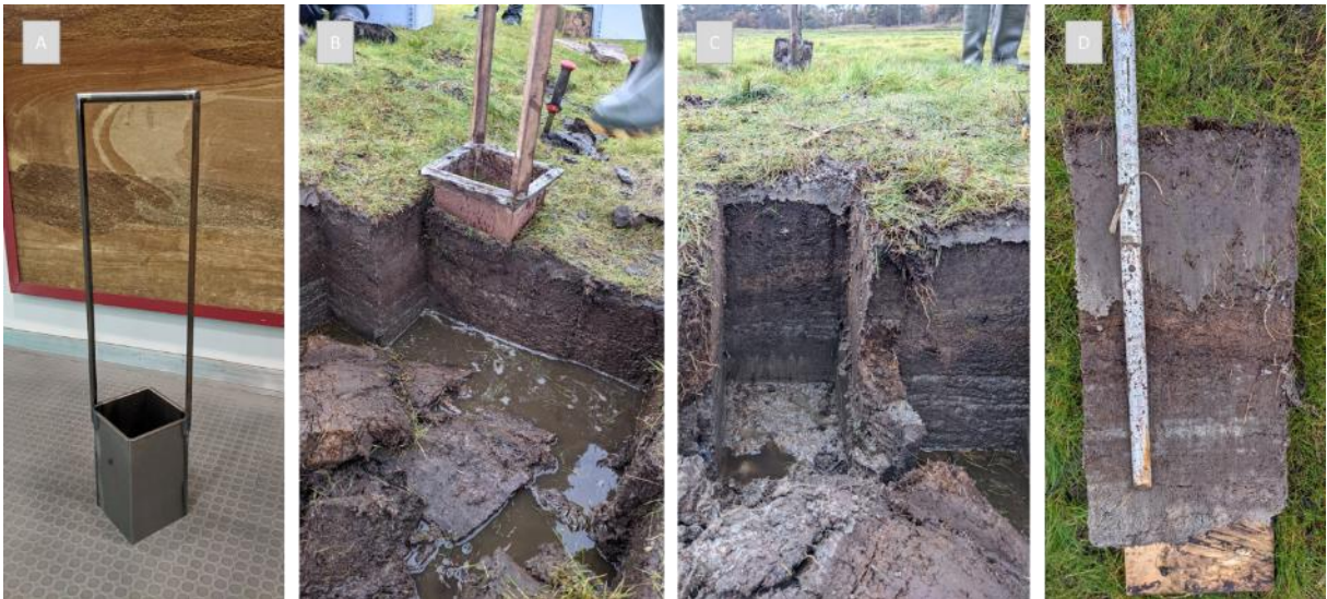
Picture S.2: Overview of the sampling procedure of individual soil sods. A shows the tailor-made square corer (20 x 20 x 35 cm). B inserted into the marsh soil. C showing the clean cut and D one individual core before cutting it to 30 cm length. Photos: Simon Thomsen (A), Ella Logemann (B-D)
