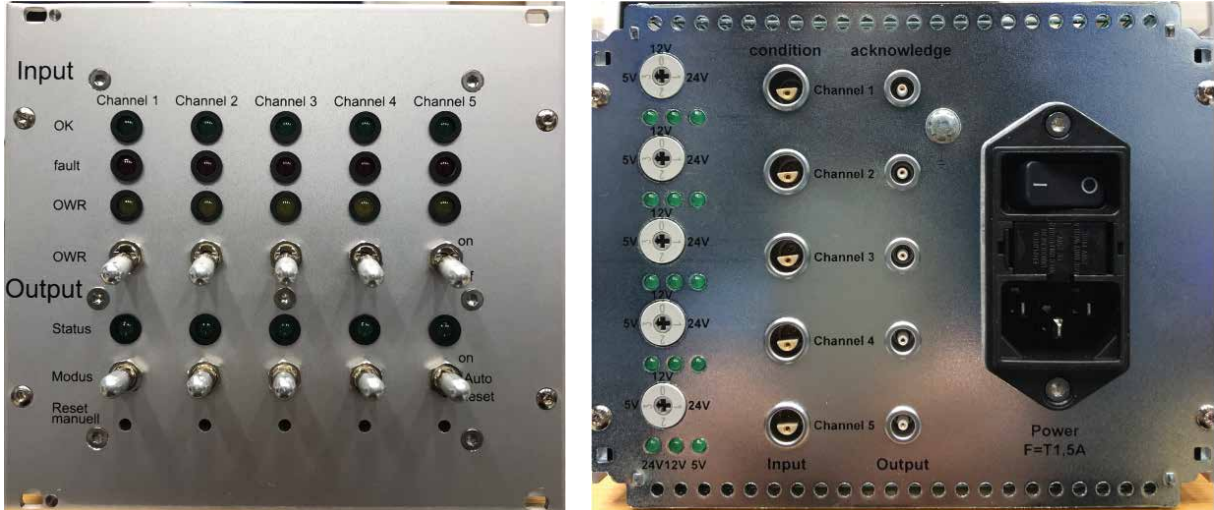
Figure A.3.: Front- (left) and back-panel (right) of the interlock controller.
