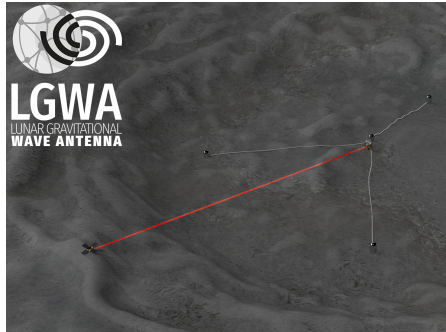
Figure 1.11: Star-like deployment configuration of four LGWA seismic stations in a kilometer-scale array. A laser-power beaming system is shown as a possible power system. (Image credit: [68]).
