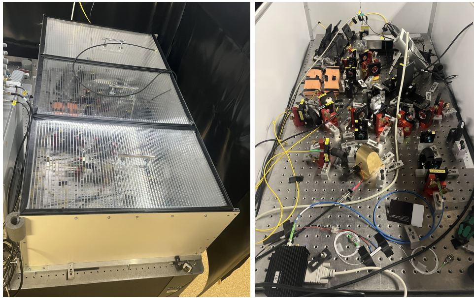
Figure 4.3: The setup in the ZOQ with the self-built housing. Left side with covers closed, right side with covers open. In the upper left corner, the polarization control is visible.
