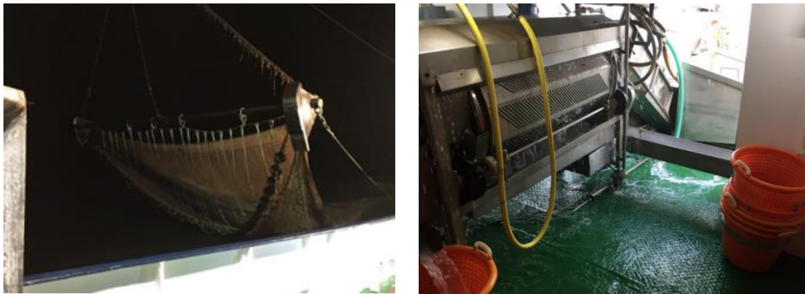
Figure 5: Beams of a brown shrimp cutter (left) and drum sieve for catch sorting (right), Photos by the author.
