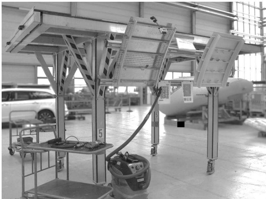
Figure 35: Mobile platform with two aircraft panels mounted at a fixed height and angle.
