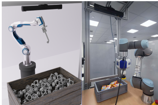
Figure 3.6: Experimental setups for robotic grasping: (left) model-based approach; (right) half-model-based approach.
