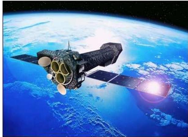
Figure 1.12: An artistic view of XMM-Newton. The satellite has a length of 10 m, a span of 18 m, a weight of 18 t and an orbiting time of two days.
