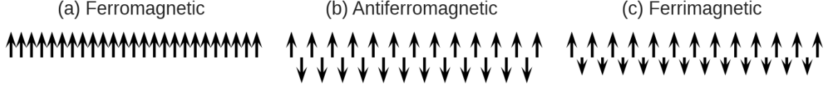
Figure 2.1: Magnetic ordering of magnetic moments in a 1D lattice. (a) Parallel arrangement giving rise to ferromagnetic materials. (b) Antiparallel arrangement which leads to antiferromagnetic materials. (c) Antiparallel with unequal magnitude which makes ferrimagnetic materials.
