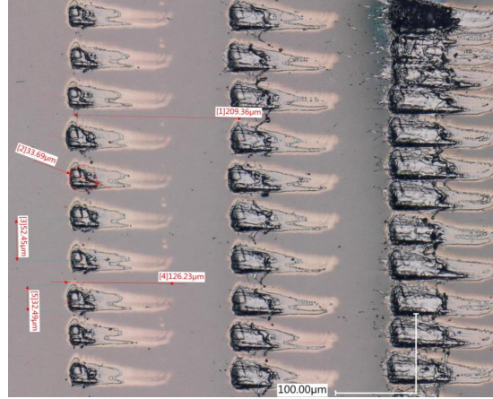
Figure 3.6: Post-exposure optical microscope image of the surface of the sample. The interaction of the X-ray with the sample locally destroys the surface leaving a crater. The 3 vertical lines are measured at different intensities, which shows in the different sizes of the craters.
