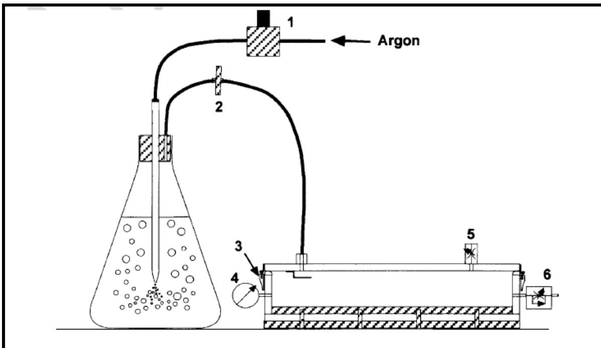
**Figure 2.1.** Scheme of the ischemia chamber used. Pressure of argon entering the gas-washing flask is controlled by a one-way flow control valve (1). The humidified gas is sterile-filtered (2). The box is constructed of Makrolon plates with two aluminum plates on the bottom (striped); it can be tightly closed by toggle latches (3), displays a pressure gauge (4), a safety valve (5) and a quick coupling socket (6) (Lewerenz, Thomsen et al. 2004).
