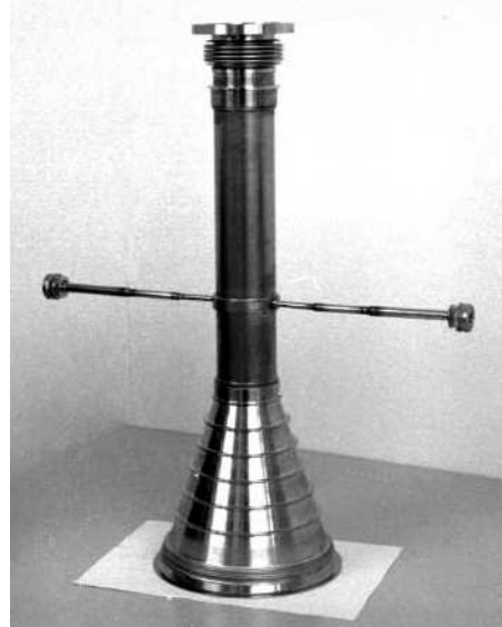
Figure 2.11: The central scattering chamber made out of 1.2 mm beryllium, with the thin tube for pellet entry and exit.
