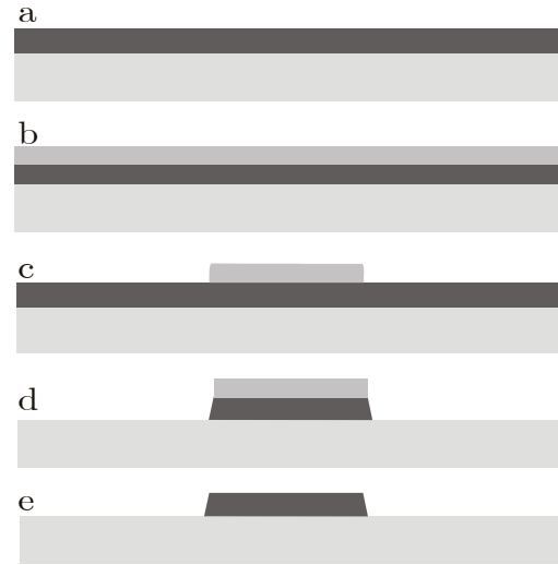
Figure 6.14: Scheme of the \text{Ar}^+ -beam etching process: (a) \text{Y}_2\text{O}_3 PLD-film is deposited, (b) photoresist is deposited on top; (c) photoresist is exposed through a mask and developed; (d) \text{Y}_2\text{O}_3 is etched with \text{Ar}^+ -beam; (e) photoresist is removed.
