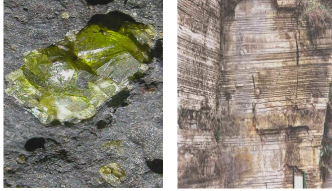
Figure 3.1: Examples for anisotropy in real rocks. Left: Olivine, anisotropy caused by preferred orientation of crystals; Right: Thin-bed layered structure.
