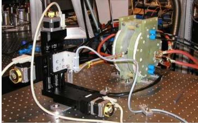
Figure 3.10: Stepper motor setup for magnetic field scans
