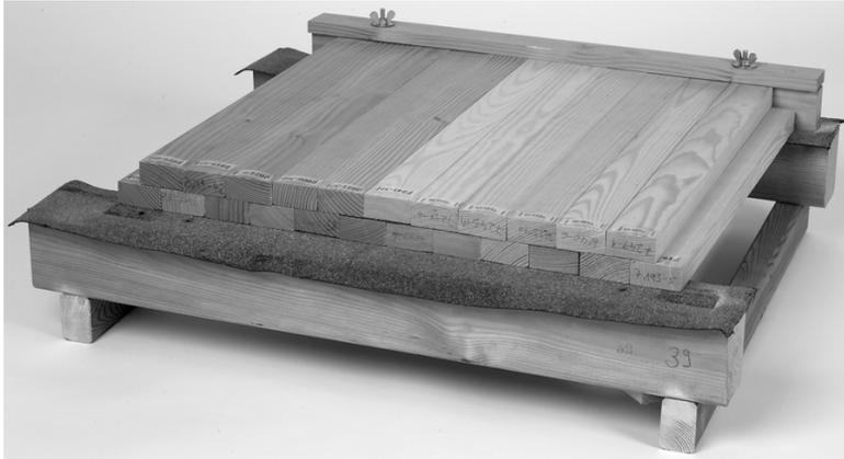
**Figure 7.2-1. Samples in horizontal double layer, shifted by one sample half to create an artificial water trap.**
