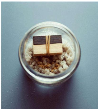
**Figure 8.2-3. Methods of test with *Reticulitermes grassei* - repellence test.**
