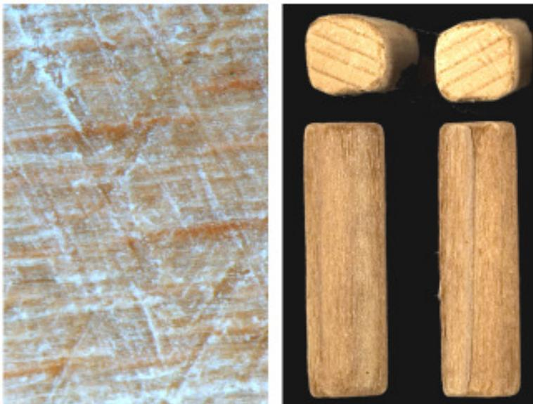
Figure 7.3-3: Abrased specimens: left: surface of a heat treated beech specimen after 1000 rounds in the Taber abraser (x10); right: heat treated silver fir specimens after 72 h abrasion in the shaker
