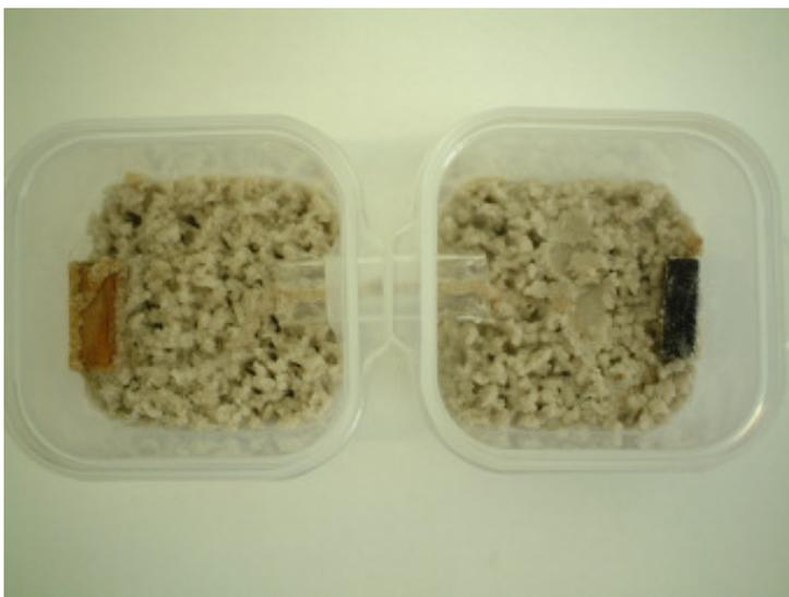
**Figure 8.2-2. Methods of test with *Reticulitermes grassei* - choice test**
