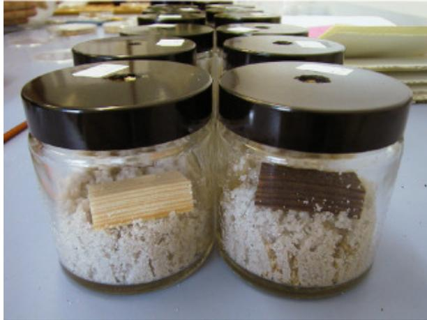
**Figure 8.2-1. Methods of test with *Reticulitermes grassei* - durability test**
