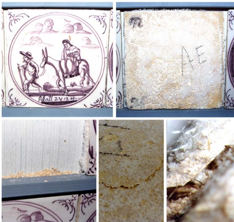
Figure 1: Dutch tin glazed tiles (18th century) in the display case: efflorescences and damage.
