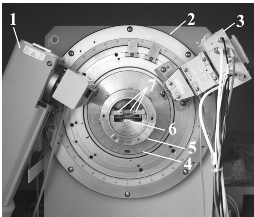
Figure 1: Front view of the open environmental chamber fixed to the \theta -circle of the D5000 diffractometer: (1) X-ray tube, (2) goniometer, (3) position sensitive detector, (4) flange (5) chamber wall (thermostated), (6) spring mounted sample holder (thermostated), (7) adjusting screws.
