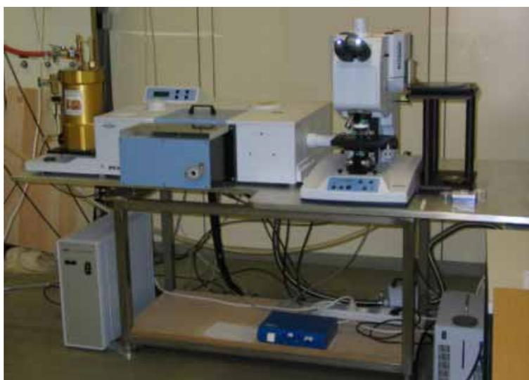
Fig. 17. Bruker 66v/S FTIR spectrometer equipped with a Bruker IRscope II microscope with a Ge ATR crystal objective and a liquid N<sub>2</sub>-cooled MCT midband detector.
