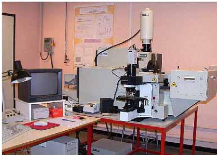
Fig. 16. Horiba Jobin-Yvon T64000 Raman Microspectroscopy.
