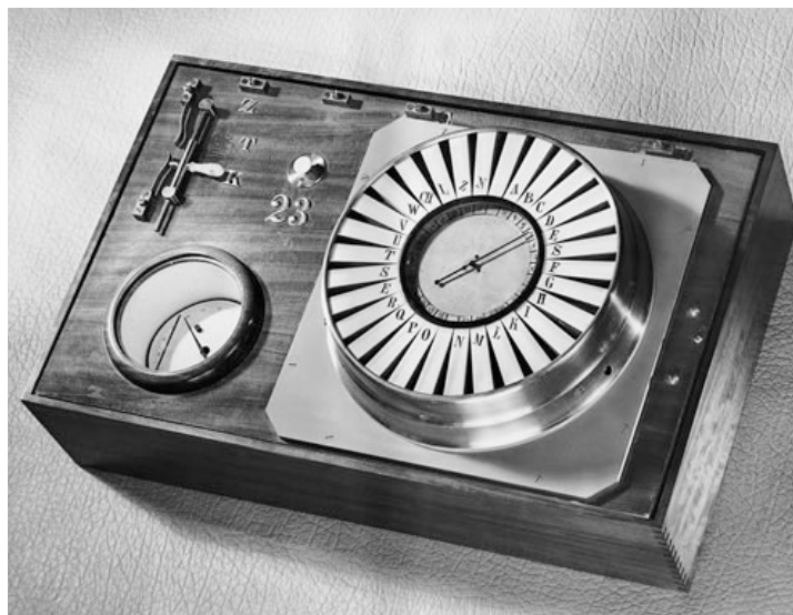
Figure 30: ‚Zeigertelegraph‘ designed 1846 by Werner von Siemens, built by Johann Georg Halske.
