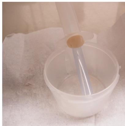
Figure 3.2 Sample in polypropylene tube for Ca leaching analysis.
