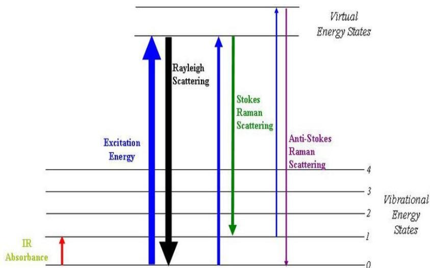
Figure 3.10 Differences in mechanism of infrared and Raman spectroscopy.
