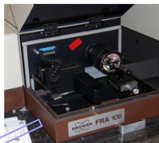
Figure 3.13 Bruker IFS 66 FTIR spectrometer equipped with a Bruker FT-Raman module FRA 106.
