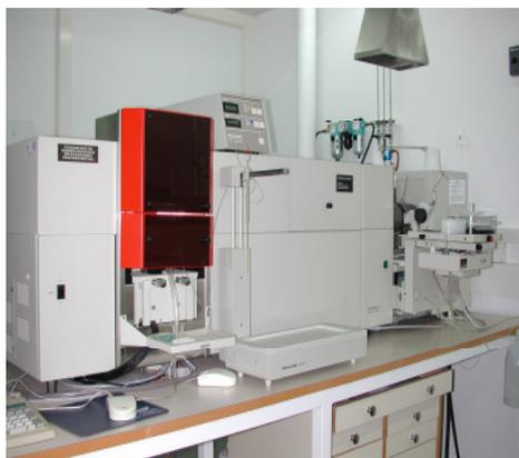
Figure 3.17 Flame atomic absorption spectrometer (FAAS).
