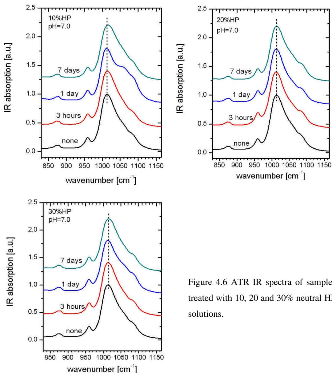
Figure 4.6 ATR IR spectra of samples treated with 10, 20 and 30% neutral HP solutions.
