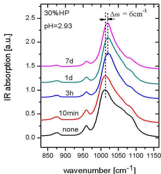
Figure 4.5 ATR IR spectra of samples before (none) and after 10 minutes, 3 hours, 1 day and 7 days treated with 30% HP solution ( $\text{pH} = 2.93$ ).
