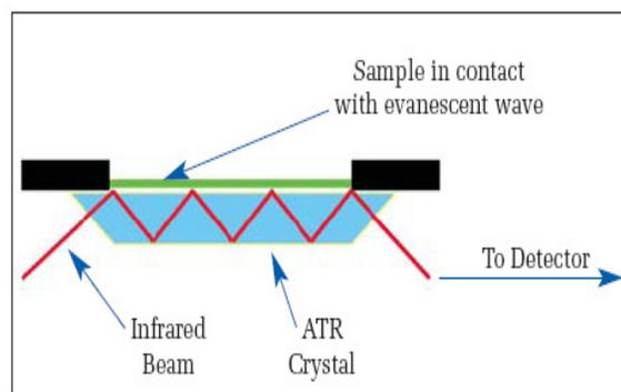
Figure 3.11 A multiple reflection ATR system.
