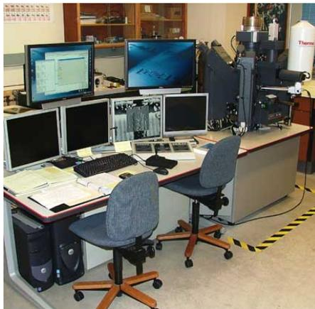
Figure 3.9 Cameca Microbeam SX100 electron microscope.
