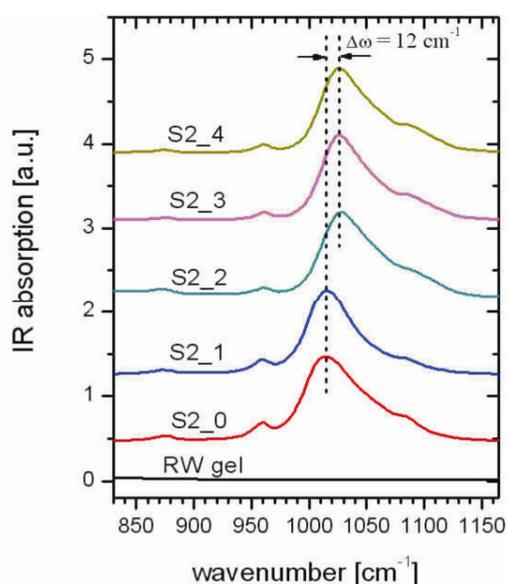
Figure 4.7 ATR IR spectra of Rapid White “whitening gel” itself, unbleached enamel (S2\_0), enamel treated with “accelerator” (S2\_1), with “whitening gel” (S2\_2), with two-step Rapid White twice daily (S2\_3) and 4 times daily (S2\_4), respectively.
