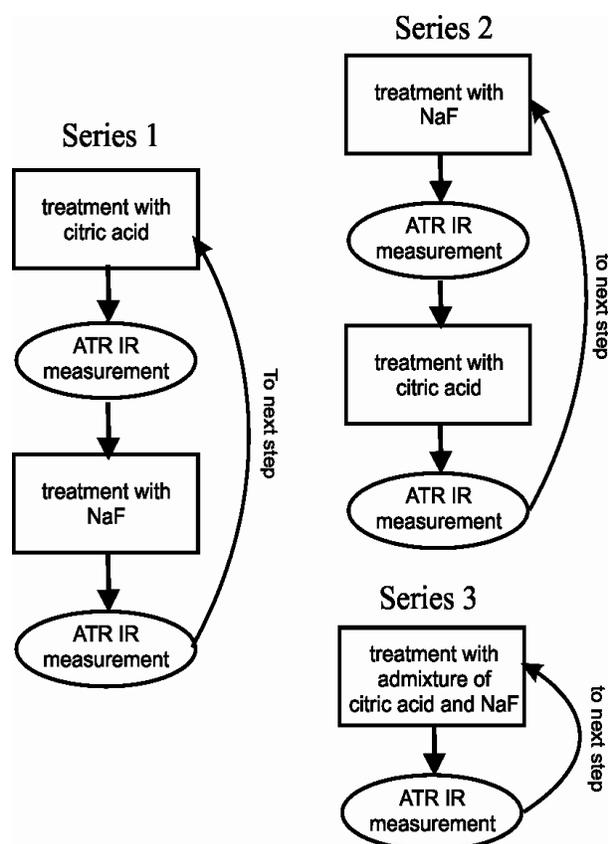
Figure 3.6 Sketch of a single step treatment for Series 1, 2 and 3, respectively.
