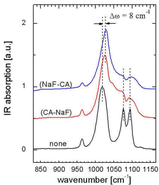
Figure 4.22 ATR IR spectra of geological hydroxyapatite (HA) treated with 0.1 mol/l citric acid solution for 10 minutes followed by a 10 minute-treatment with 1.0% NaF solution (CA-NaF), and with 0.1 mol/l citric acid solution for 10 minutes after a 10 minute-treatment with 1.0% NaF solutions (NaF-CA). Both treatments were repeated 14 cycles.
