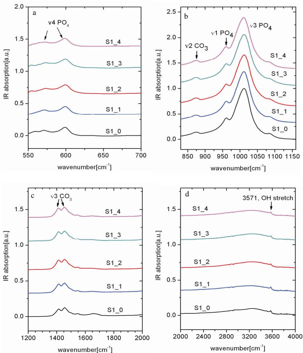
Figure 4.4 ATR IR spectra of samples treated with Opalescence Xtra Boost for recommended exposure time (S1\_1) and prolonged time (S1\_2), Opalescence PF 20% (S1\_3) and sodium perborate (S1\_4). For comparison the spectrum of unbleached enamel (S1\_0) is also included. (a) spectra in the range of 550-700  $\text{cm}^{-1}$ , (b) spectra in the range of 830-1165  $\text{cm}^{-1}$ , (c) spectra in the range of 1200-2000  $\text{cm}^{-1}$  and (d) the spectra range of 2000-4000  $\text{cm}^{-1}$ .
