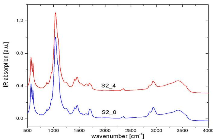
Figure 4.3 IR absorption spectra of the control group (S2\_0) and two-step Rapid White (S2\_4).
