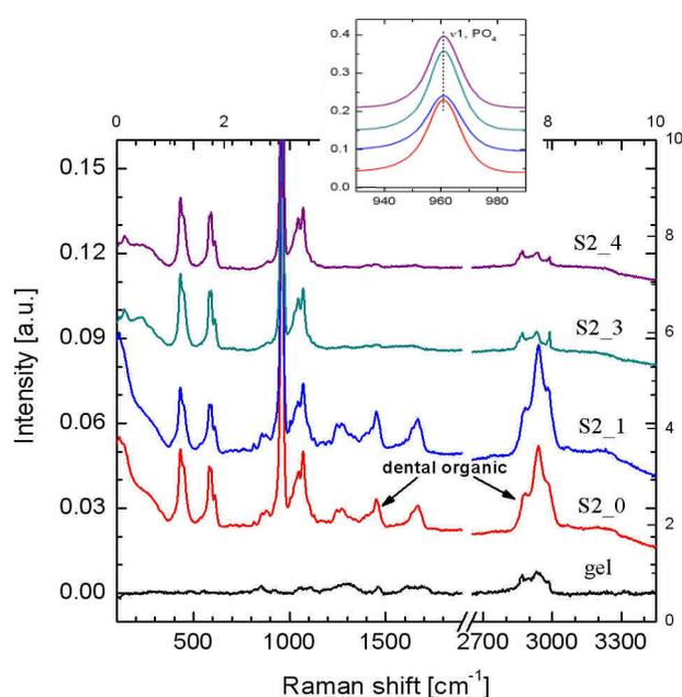
Figure 4.11 Raman spectra of samples treated with the non-peroxide-based bleaching agent (Rapid White) and the unbleached reference sample: S2\_0, unbleached; S2\_1, treated with “accelerator”; S2\_3, with two-step Rapid White twice daily and S2\_4, with two-step Rapid White 4 times daily. The insert shows details of the  $\nu_1$   $\text{PO}_4$  mode.
