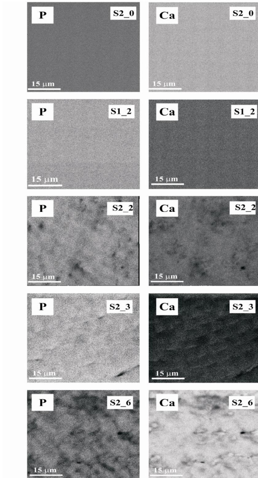
Figure 4.13 Electron-probe P- and Ca-mapping of enamel unbleached (S2\_0), treated with Opalescence Xtra Boost (S1\_2), with Rapid White "whitening gel" (S2\_2), with two-step Rapid White (S2\_3) and 0.1 mol/l citric acid solution (S2\_6) for 7 days, 2x10 min per day.
