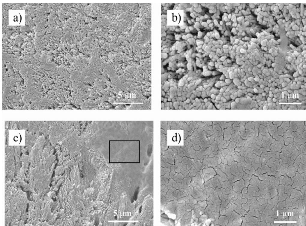
Figure 4.20 SEM micrographs of enamel treated with 0.1 mol/l citric acid solution for 10 minutes (a, b) and enamel firstly treated with (0.1 mol/l citric acid + 0.5% NaF) solution for 14×10 min and then immersed in 0.1 mol/l citric acid solution for 10 minutes (c, d). The magnification for (a) and (c) is 5 000×, while for (b) and (d) it is 20 000×; the rectangular frame in (c) marks the area from which the micrograph in (d) was taken.
