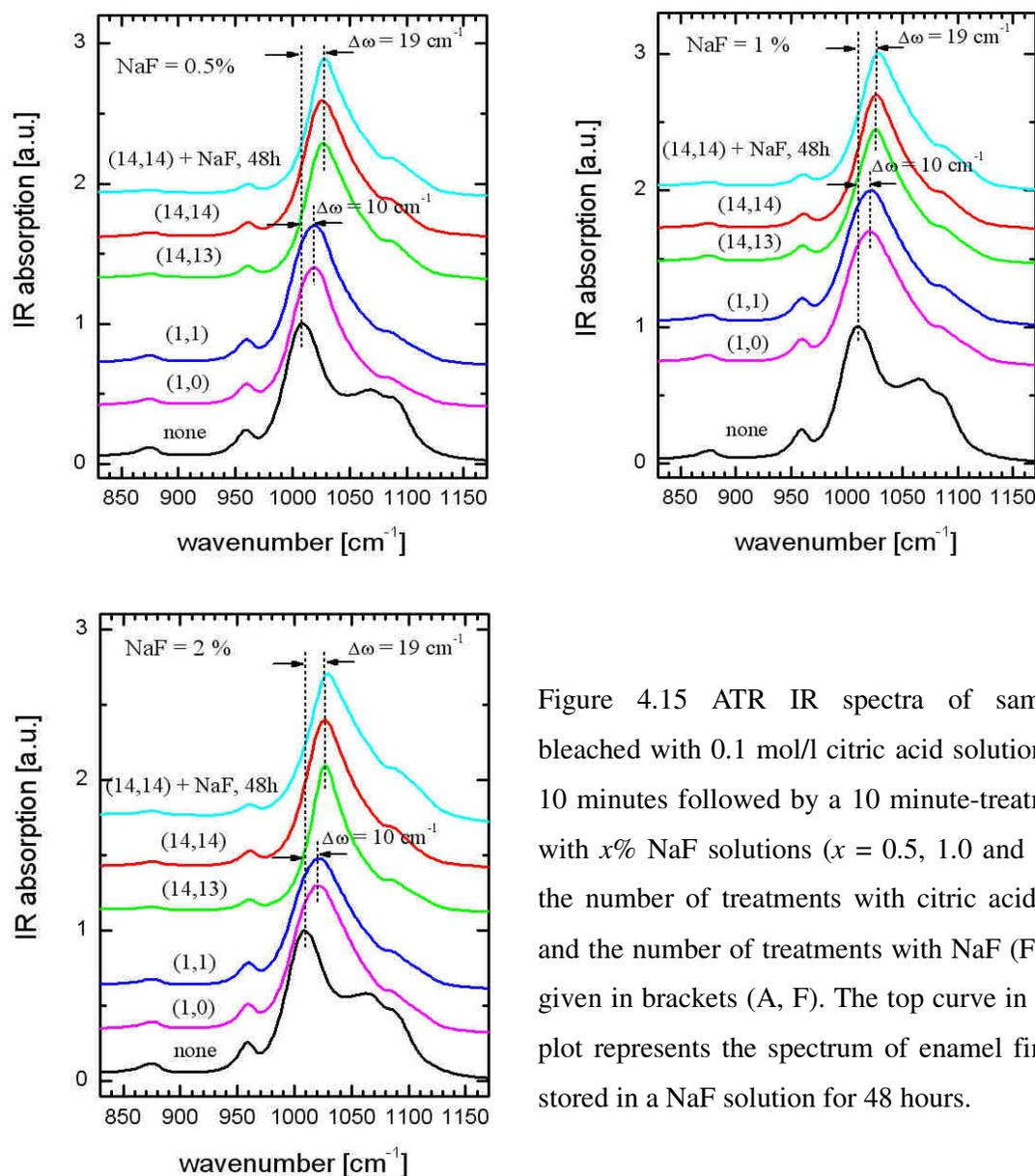
Figure 4.15 ATR IR spectra of samples bleached with 0.1 mol/l citric acid solution for 10 minutes followed by a 10 minute-treatment with  $x\%$  NaF solutions ( $x = 0.5, 1.0$  and  $2.0$ ); the number of treatments with citric acid (A) and the number of treatments with NaF (F) are given in brackets (A, F). The top curve in each plot represents the spectrum of enamel finally stored in a NaF solution for 48 hours.
