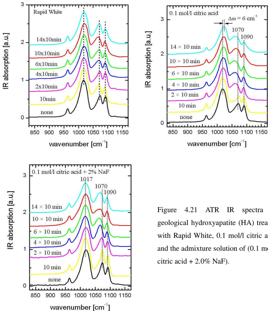
Figure 4.21 ATR IR spectra of geological hydroxyapatite (HA) treated with Rapid White, 0.1 mol/l citric acid and the admixture solution of (0.1 mol/l citric acid + 2.0%  $\text{NaF}$ ).
