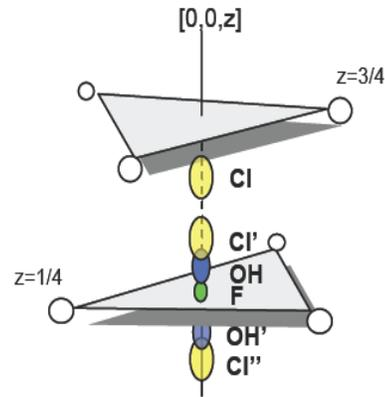
Figure 2.5 Possible anion positions in the channel inside the HA unit cell.
