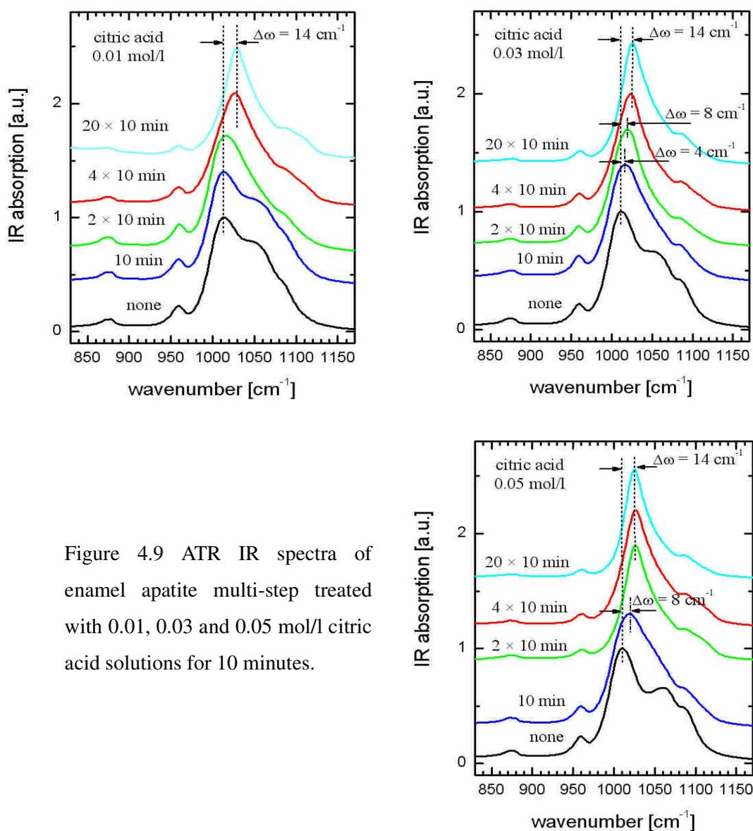
Figure 4.9 ATR IR spectra of enamel apatite multi-step treated with 0.01, 0.03 and 0.05 mol/l citric acid solutions for 10 minutes.
