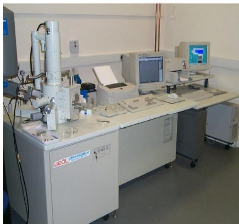
Figure 3.8 JEOL 5600LV scanning electron microscope.
