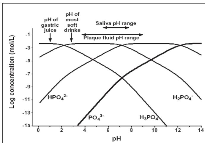
Figure 2.7 The effect of pH on the concentrations of the various inorganic phosphate species in saliva containing a total phosphate concentration of  $5 \times 10^{-3}$  mol/l. There is a marked fall in the concentration of  $\text{PO}_4^{3-}$  (thick line) as the pH value is reduced [Dawes, 2003].
