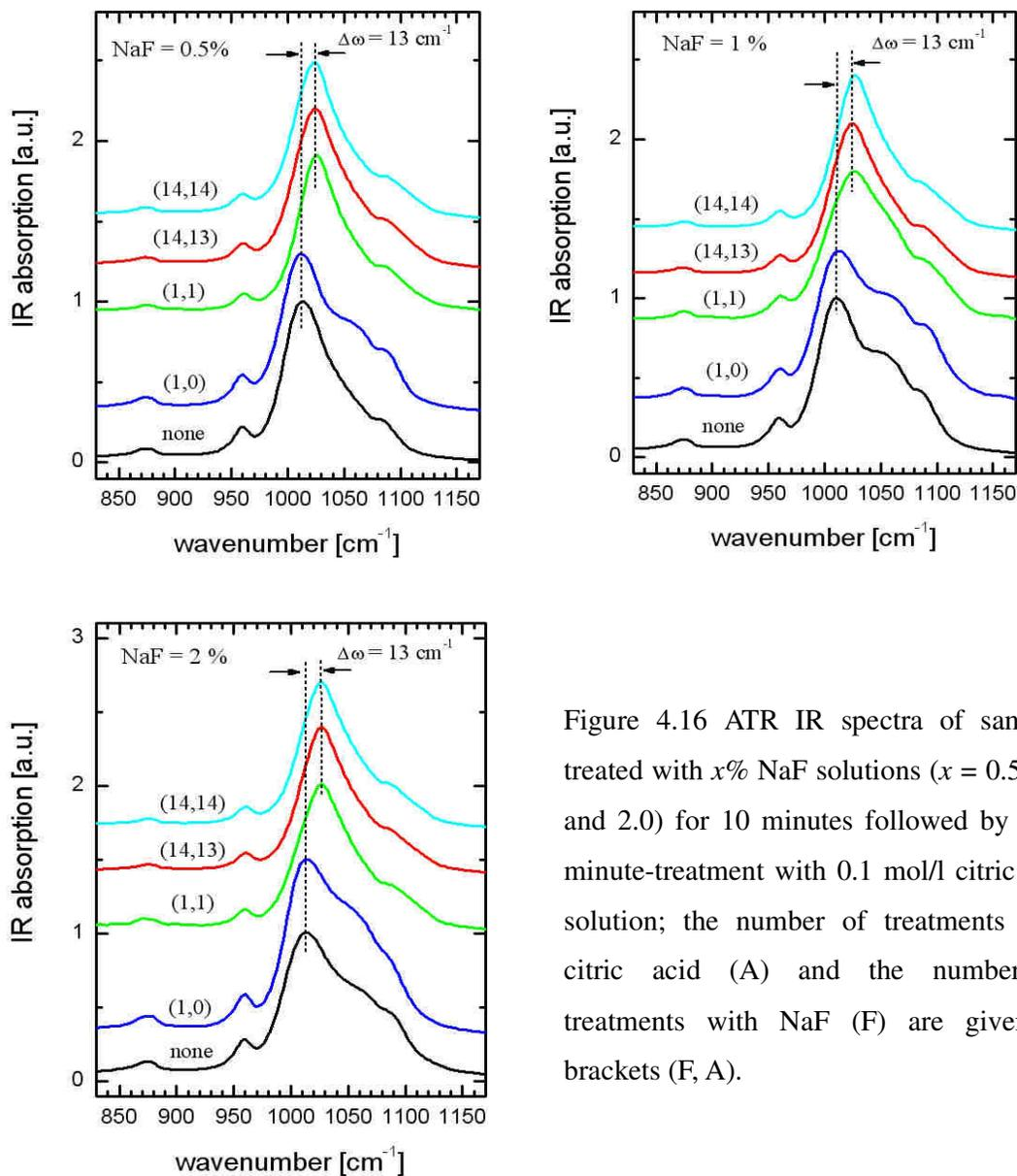
Figure 4.16 ATR IR spectra of samples treated with  $x\%$  NaF solutions ( $x = 0.5, 1.0$  and  $2.0$ ) for 10 minutes followed by a 10 minute-treatment with  $0.1 \text{ mol/l}$  citric acid solution; the number of treatments with citric acid (A) and the number of treatments with NaF (F) are given in brackets (F, A).
