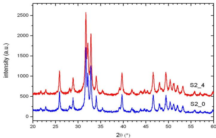
Figure 4.2 XRD patterns of the control group (S2\_0) and two-step Rapid White (S2\_4).
