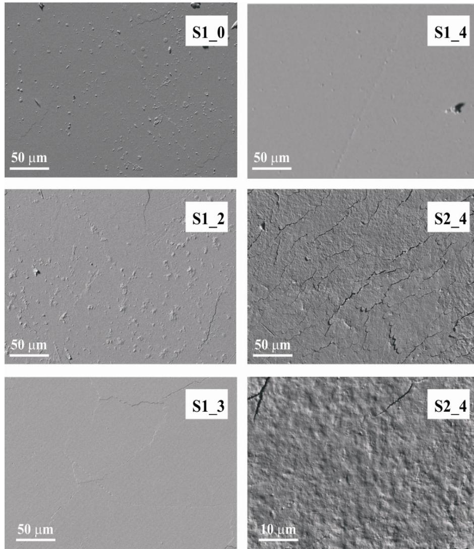
Figure 4.1 SEM micrographs of samples S1\_2, S1\_3, S1\_4 and S2\_4 treated with Opalescence Xtra Boost (3h), Opalescence PF 20%, sodium perborate and sodium chlorite-based Rapid White, respectively. For comparison the SEM micrograph of unbleached enamel (S1\_0) is also included; the micrograph of S2\_4 is given in two different magnifications (see scale bars).
