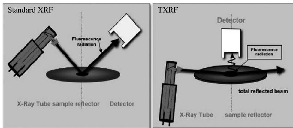
Figure 3.16 Comparison between conventional (left) and total reflection mode of excitation (right).
