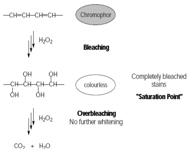
Figure 2.11 Illustration of the chemical oxidation reaction of dye molecules comprising unsaturated double bonds with HP to colorless molecules. After conversion of all stains to colorless products the saturation point is reached. Further bleaching would merely cause degradation to carbon dioxide ( $\text{CO}_2$ ) and water ( $\text{H}_2\text{O}$ ) but would not increase the whitening effect (overbleaching).
