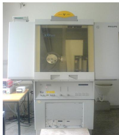
Figure 3.15 Philips X'pert diffractometer.
