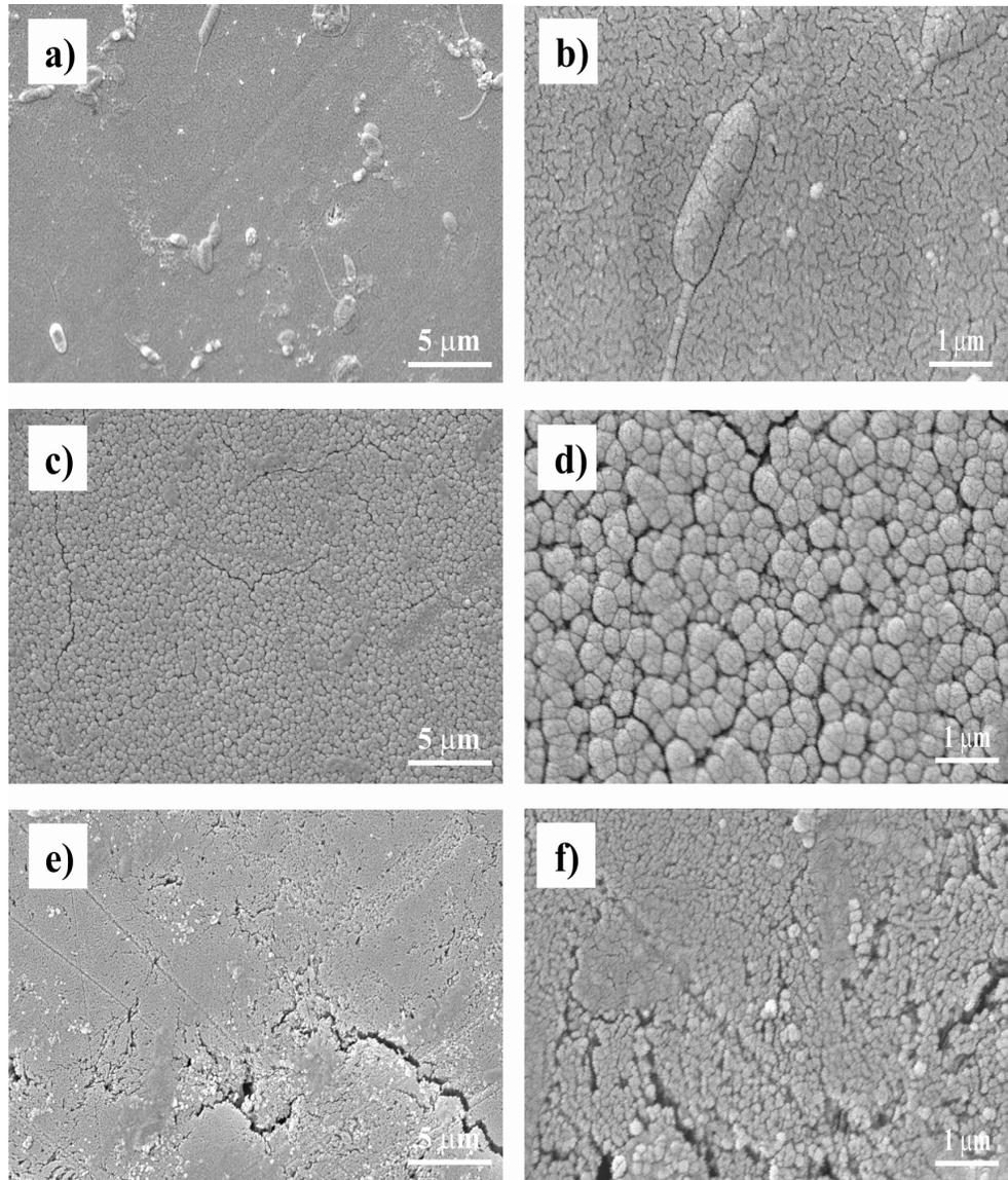
Figure 4.19 SEM micrographs of untreated enamel (a, b), enamel treated for 14 cycles of 10 minutes with (0.1 mol/l citric acid + 1.0% NaF) solution (c, d) and treated for 14 cycles of 10 minutes with (0.1 mol/l citric acid + 2.0% NaF) solution (e, f). The magnification for (a), (c) and (e) is 5 000 $\times$ , while for (b), (d) and (f) it is 20 000 $\times$ .
