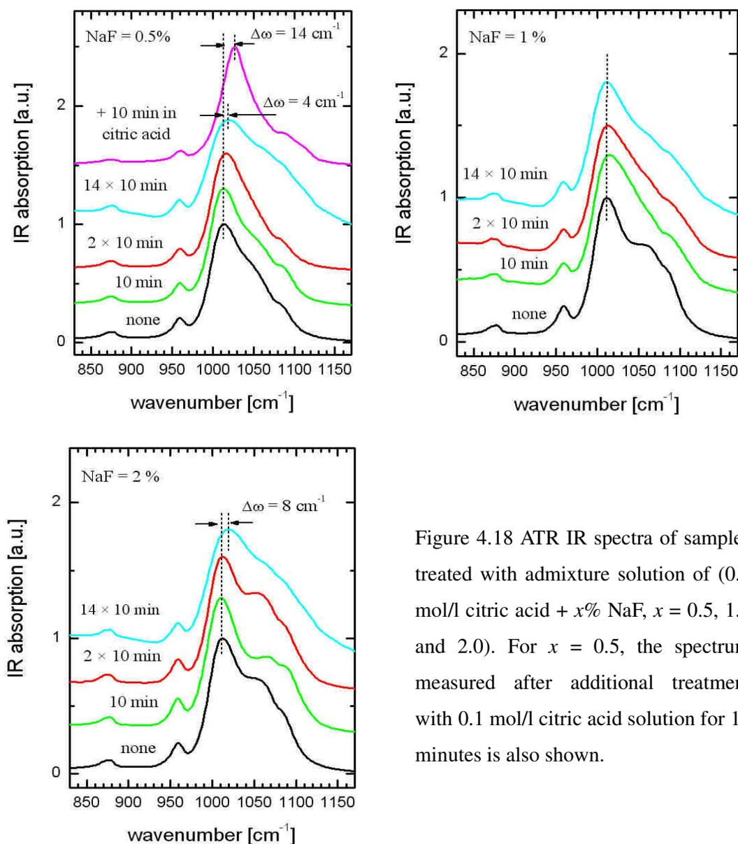
Figure 4.18 ATR IR spectra of samples treated with admixture solution of (0.1 mol/l citric acid +  $x\%$  NaF,  $x = 0.5, 1.0$  and  $2.0$ ). For  $x = 0.5$ , the spectrum measured after additional treatment with 0.1 mol/l citric acid solution for 10 minutes is also shown.
