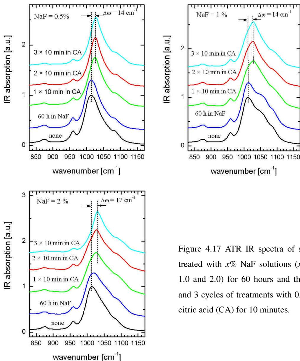
Figure 4.17 ATR IR spectra of samples treated with  $x\%$  NaF solutions ( $x = 0.5, 1.0$  and  $2.0$ ) for 60 hours and then 1, 2 and 3 cycles of treatments with 0.1 mol/l citric acid (CA) for 10 minutes.
