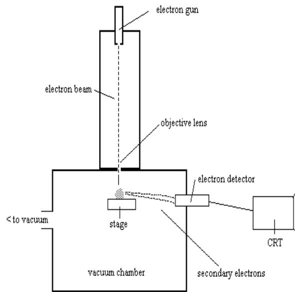
Figure 3.7 Schematic drawing of a generic SEM.
