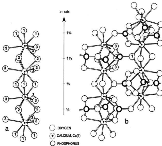
Figure 2.4 (a) Oxygen coordination of columnar Ca1 ions in apatite. (b) Columns linked via PO<sub>4</sub> tetrahedra. The oxygen atoms in (a) and in one tetrahedron in (b) have been numbered, and positions of the horizontal mirror planes at 1/4, 3/4 etc. are marked on the c-axis [Beever and McIntyre, 1946].
