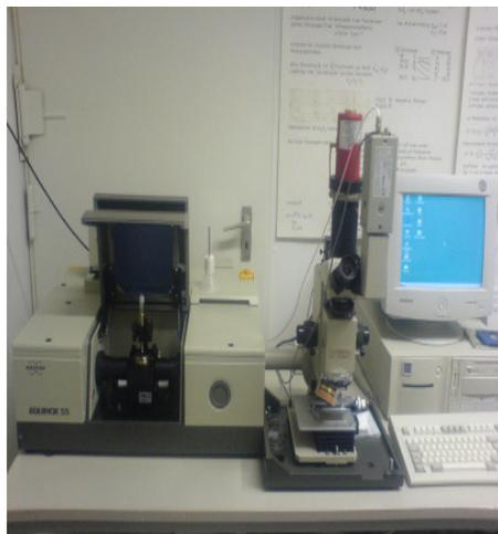
Figure 3.12 Bruker Equinox 55 FTIR spectrometer equipped with a Pike MIRacle ATR accessory.
