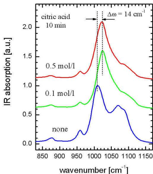
Figure 4.8 ATR IR spectra of enamel treated with 0.1 and 0.5 mol/l citric acid solutions for 10 minutes.
