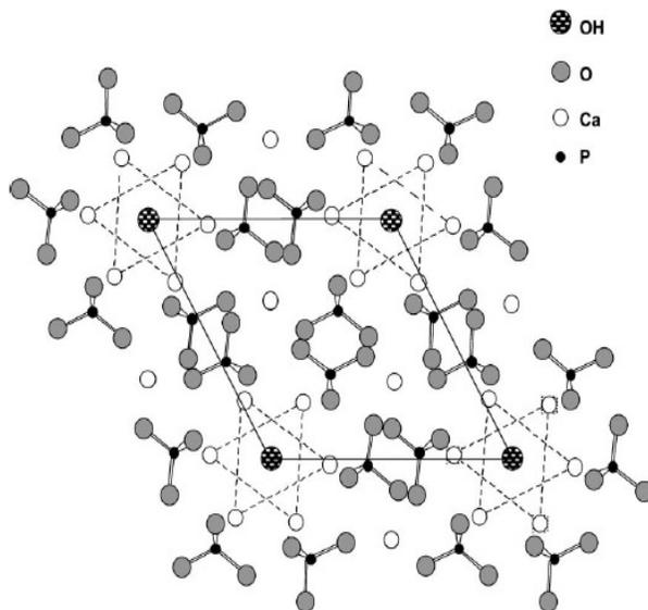
Figure 2.3 Sketch of the hydroxyapatite (HA) structure. View along the  $c$ -axis showing  $\text{PO}_4$  tetrahedral ionic groups, Ca-ions and “channel ions”. Parallelogram indicates HA unit cell. Six Ca atoms form a six-fold site (indicated by dashed lines) in which the channel ions reside ( $\text{OH}^-$  in the case of HA). These channels are oriented along the viewing direction.
